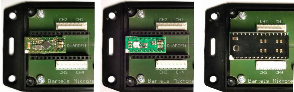
Use caution when removing the pump driver from the board in order to not bend the pins of the chip. IC pliers are recommended to be used for extraction.
