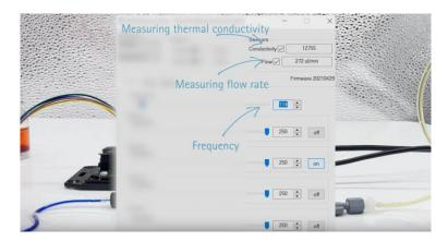
Which makes sense, as the viscosity is way different from water. In order to optimize the pump rate, we increase the frequency. This leads to a further decrease of the pump rate. This means that the optimized frequency has to be lower. We use the SLF3C-1300F sensor to take a reading of the thermal conductivity and find it to be 7'500 a.u. this indicates that we have the glycerin/water mixture in our sensor and pump. We can clearly differentiate between the two liquids (water and water/glycerin).
