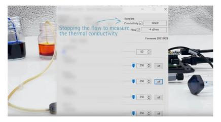
Next, we use a much higher frequency. It shows that the pump rate remains low. This indicates that our frequency is now too high. The water is not able to follow the rapid pump strokes. We therefore lower the actuation frequency of the pump a little bit and with this, hit the maximum pump rate. This frequency could also be saved in a look-up table as the optimum actuation frequency for pumping liquids that mainly contain water.
