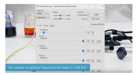
Afterwards we switch to a different liquid. A mixture between glycerin and water with a viscosity of 18 mPas. We use the same actuation frequency for the pump we found to be optimal with water. It shows that we achieve a very low pump rate.
