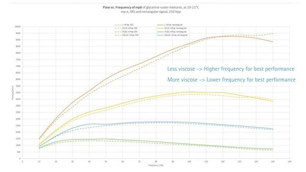
So, again, the shear stress counteracts the force of the piezo actuator, increasing the frequency would mean to increase a counteracting force of the piezo force which leads to a lower pump performance although the driving parameters (frequency) of the pump are increased.
