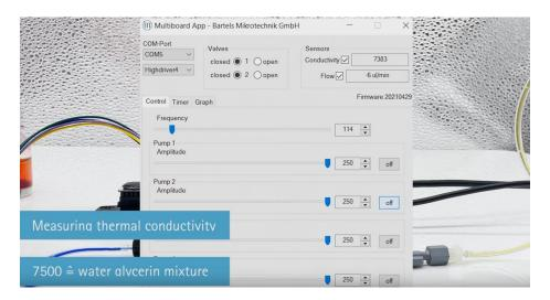
We lower the actuating frequency and find the maximum pump rate at 50 Hz. We have now determined the optimal pump actuation frequency of water and our water-/glycerin mixture.
