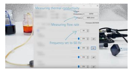
We then stop the flow and take a reading with the SLF3C-1300F. It gives us a value of 10'500 a.u. given the fact that we did not implement a temperature compensation for this experiment, this value is close enough to the calibrated value for water (10'000 a.u.) to identify the liquid in the pump as being water.
