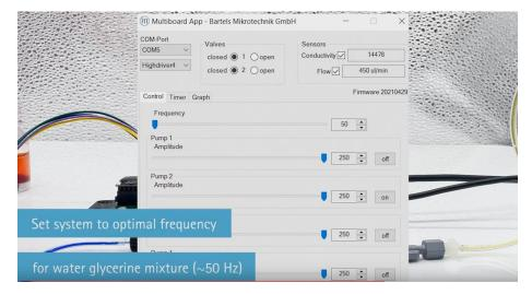
For future experiments we can identify with the SL3C-1300F-sensor with liquid is present in our system and choose the optimal pump frequency accordingly with a look-up table.
