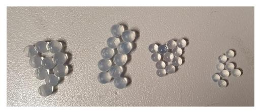
Figure 3 Generated Alginate beads; From left to right: 3.75 mm, 3 mm, 2.6 mm, 2.5 mm in diameter
