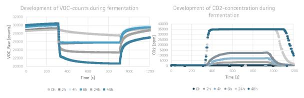
It shall be noted that high VOC-concentrations correspond to low count rates by the SGP40 sensor because the sensor is observing the degree of air quality, hence the inverse of pollution levels. Moreover, the  $CO_2$  concentration is directly given in ppm while the VOC-sensor only provides count rates, whose quantitative
