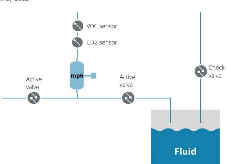
To verify whether differences in gas concentrations can be detected after passing through the mp6 micropumps, a reservoir including a sealed lid with four ports is utilized.
