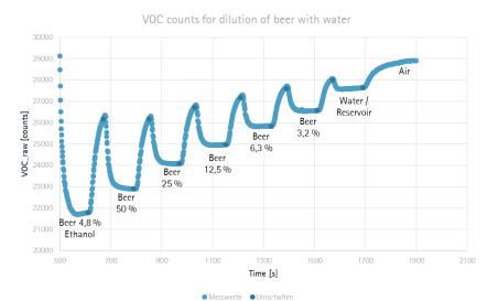
In conclusion,  $CO_2$  as well as VOC concentrations rise with advanced fermentation. That way, by simply assigning a reference (e.g. beer with 4.8%  $C_2H_5OH$ ), the fermentation process of yeast into beer can be protocolled industrially with very little space and resources needed. Since all data can be obtained via gas phase analysis, contaminants are mostly excluded from the measurement.
