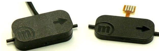
Figure 1: Sample of a mp6 with integrated electronics (left hand) and a single mp6 (right hand)
