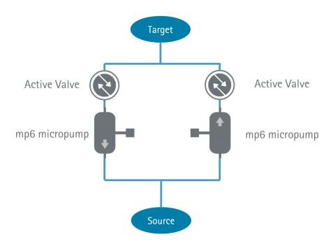
Figure 10 Block diagram for using two micropumps in opposite direction and two 2/2-way valves
