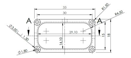
Figure 12 Dimensions of the mounting frame mp-mf
