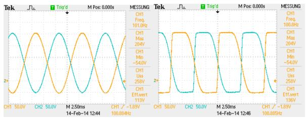
Figure 15 Scopeshots of a mp6 micropump at 250Vpp; 100 Hz; sine signal (left); SRS signal (right) / Voltage at piezo actuator 1 ≜ CH1 & piezo actuator 2 ≜ CH2
