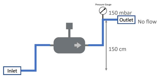
Figure 3 Example increased pressure due to height difference in the system
