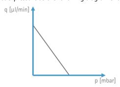
Figure 2 General dependency flow rate/ backpressure
