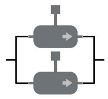
The following diagrams prove the fact that pumps in series or respective in parallel increase the pressure or flow rate:
