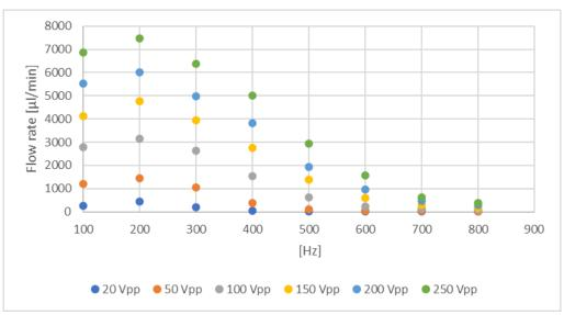
Figure 12 Example mp6 run by mp-Highdriver pumping water (high frequencies)
