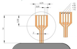
Figure 16 Schematic of the FCC connector of the mp6 micropump; all dimensions in [mm]
