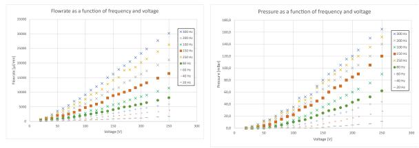
Figure 7 Typical mp-Labtronix flow rates for water (top left), water pressure (top right), flow rates for air (bottom left), air pressure (bottom right)
