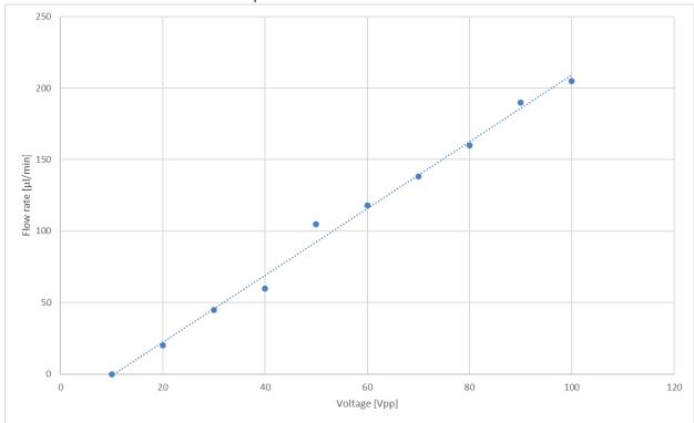
Figure 14 Flow restriction utilizing capillary I = 70 mm and ID = 65  $\mu$ m with mp-Highdriver at 50 Hz pump frequency
