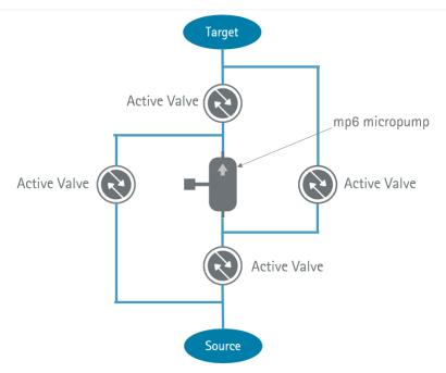
Figure 9 Block diagram for a bidirectional driven mp6 micropump, assisted by a smart combination of four Takasago valves.
