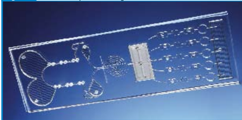
Figure 2: Microfluidic chip for mobile diagnostics. 4
