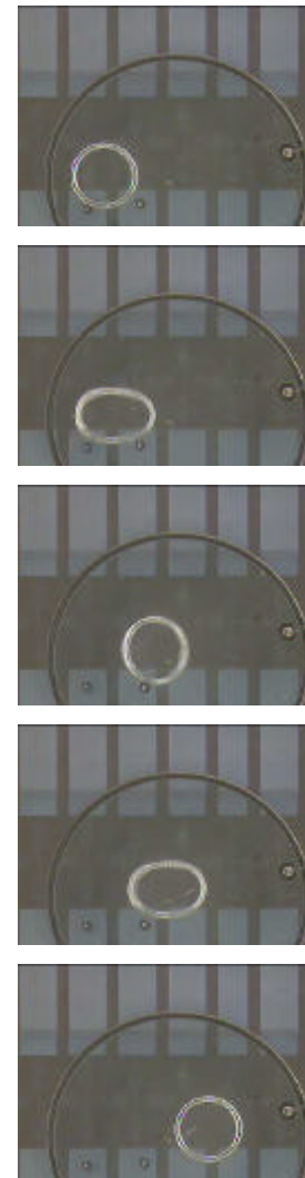
Sequence of liquid movement with electro-wetting.
