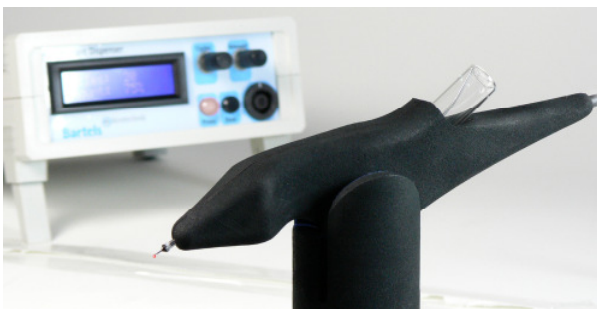
Micropump based hand dispenser for the dosing of smallest volumes
