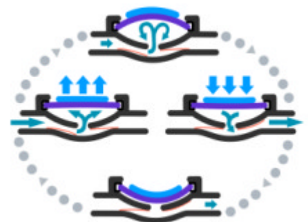
Functional principle of piezomembrane pump.
