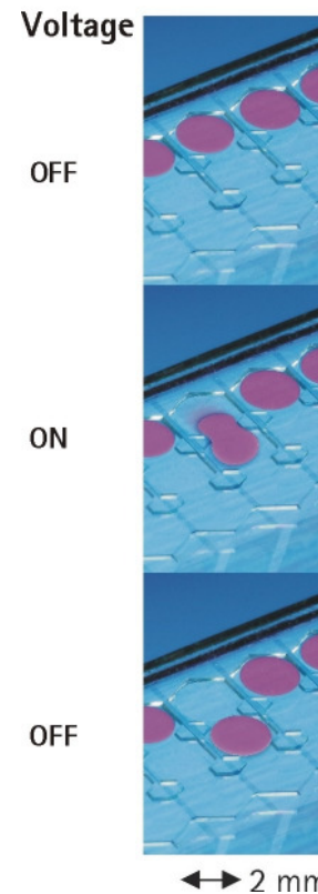
Electrowetting: A droplet is moved from one position to another when voltage is applied.
