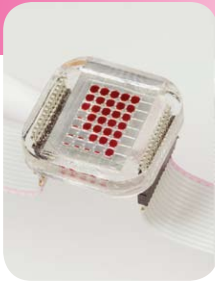
Electrowetting is used to move droplets in and out of 2 mm pixels in a 5 x 7 monochrome array that is passively driven.
