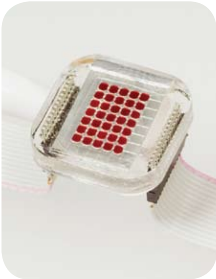
Electrowetting is used to move droplets in and out of 2 mm pixels in a 5 x 7 monochrome array that is passively driven.
