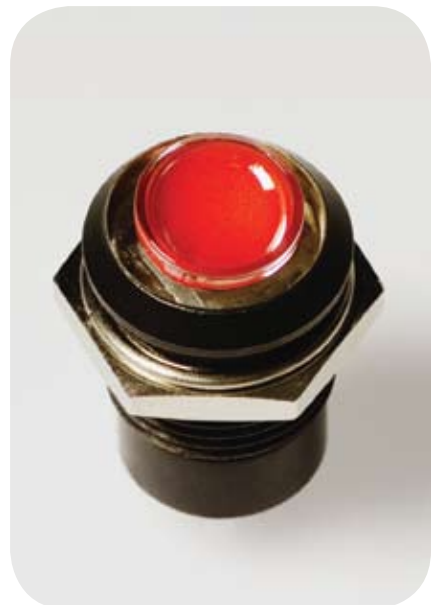
In a simple indicator implementation, electrowetting moves the colored dye in and out of the visible area under a lens, serving as an LED alternative.
