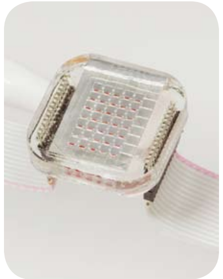
Electrowetting is used to move droplets in and out of 2 mm pixels in a 5 x 7 monochrome array that is passively driven.
